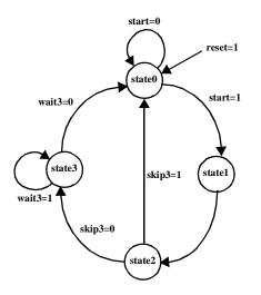
Using Macros for state definition As an alternative for**parameter** state0=0, state1=1, state2=2, state3=3; one can use macros. For example after the definition below 2'd0 will be textually substituted whenever `state0 is used. define state0 2'd0 `define state1 2'd1 `define state2 2'd `define state3 2'd3; When using macro definitions one must put a back quote in front. For example: case (state) `state0: Zot = 3'b000;`state1: Zot = 3'b101;
