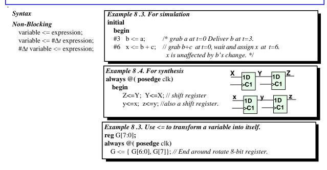
The following example shows interactions between blocking and non-blocking for simulation. Do not mix the two types in one procedure <u>for synthesis</u>.
